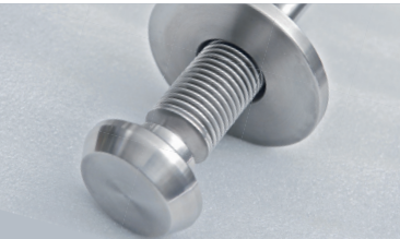
Conical sealing: No impurities remain on the sealing surface. When it tends to close, the sealing surface has a selfcleaning effect to achieve linear sealing.
